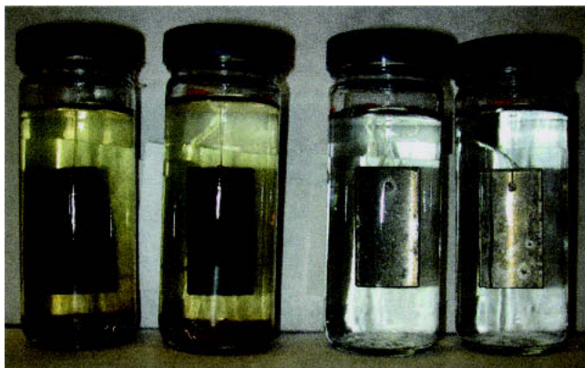
Fig. 1 Test setup for evaluating the influence of inhibitor additives on corrosion processes in seawater; sample bottles from left to right, 1018 steel in \frac{1}{4} and \frac{1}{2} strength seawater and 6061 aluminum in \frac{1}{4} and \frac{1}{2} strength seawater
